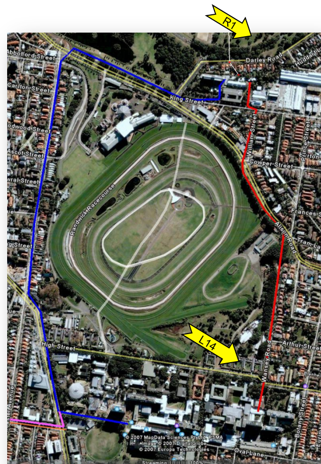
Fibre Routes from Kensington Campus to new R1 Data Centre
